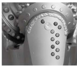
掌背金刚石复合齿占100% (D1) Diamond compound teeth on the leg accounts for 100% (D1)
