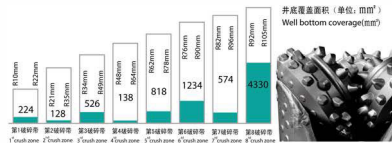
普通牙齿井底覆盖图 Well bottom cover in case of ordinary tooth
